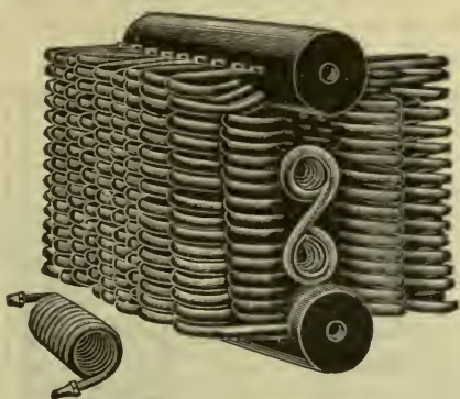
FIG. 354.—The Ofeldt water tube boiler (marine type). This boiler consists of two horizontal drums connected on each side by numerous vertical up flow coils. Between the two series of coils are a set of down flow coils connected to the two drums. The cooler water in the upper drum flows down through these coils to the lower drum, thence up through the up flow coils absorbing heat from the fire and re-entering the upper drum as steam and water.
